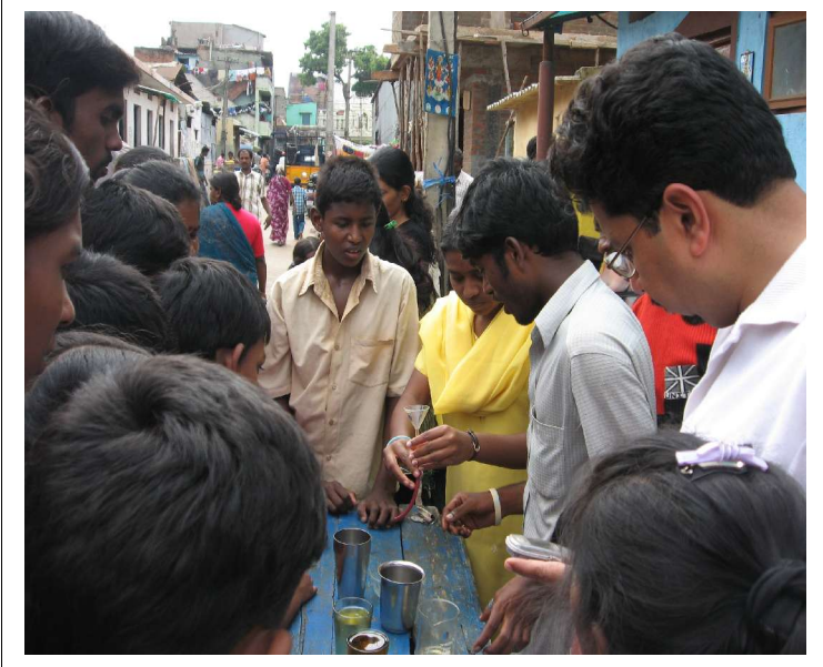
Measurement of Time: Prabhakar and partner measuring the time it takes for a given quantity of oil to flow through a funnel. AID volunteer Srimi is measuring the time
